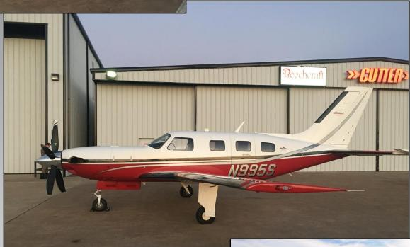
2,210 Hours Total Time | 1,054 CSN 5,134 lbs Max Ramp | Useful Load 1,684 lbs 5-Blade MT Prop Installed April 2015 - 157 Hours Since New 729 Hours Since Hot Section Inspection **Annual Inspection Complete May 2018 IFR Certification Complete May 2018**
