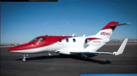
Featuring Honda Aircraft Exclusive: OTWEM – Over The Wing Engine Mounts Honda GE HF 120 Engines NLF (Natural Laminar Flow) Fuselage and Wings Composite Fuselage
