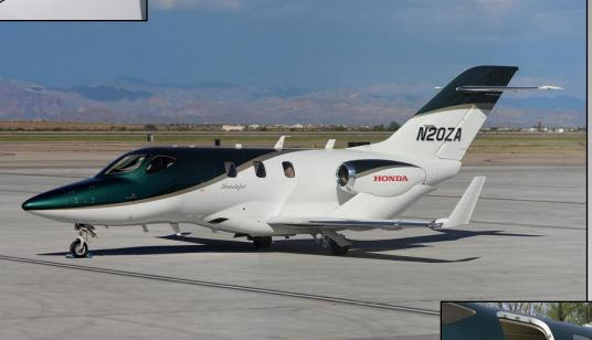
270 Hours 180 Cycles OTWEM – Over The Wing Engine Mounts Honda GE HF 120 Engines NLF (Natural Laminar Flow) Fuselage and Wings Composite Fuselage
